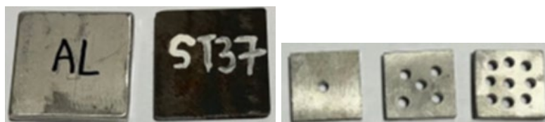
Gambar 5 Sampel (Luas Permukaan). Solid Aluminium ( 40 \text{ Cm}^2 ); Baja ST37 ( 40 \text{ Cm}^2 ); Aluminium foam 1 Lubang ( 9,22 \text{ Cm}^2 ) Aluminium foam 5 Lubang ( 7,72 \text{ Cm}^2 ); Aluminium foam 9 lubang ( 5,83 \text{ cm}^2 );
