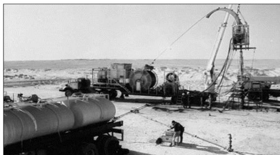
Figure 1. Matrix stimulation treatment using a coiled tubing unit, pump truck, and fluid transport ( Sumber: Economides, M and Boney, C, Reservoir Stimulation, 1989: 51)
